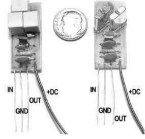
The old 455 KHz filter (photo) we once made for AM and AM/FM models is now discontinued. But the newer CBs almost always use a 10.695 MHz second or high IF; our 10.695 MHz filter can be used in them with even better results. That's because crystal filters are much sharper than the ceramic types commonly used for 455 KHz. Just be sure to <u>specify your radio model</u> when ordering it.
